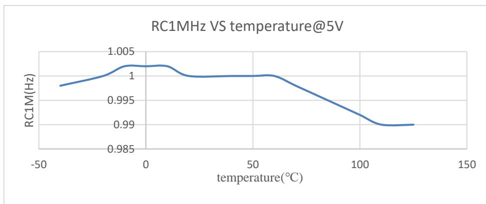
f<sub>RC1M</sub> temperature curve
