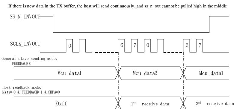
Schematic diagram of SPI continuous working in high-speed communication mode (host):
