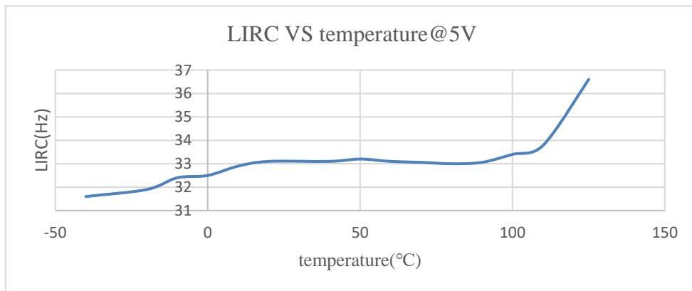
f<sub>LIRC</sub> temperature curve
