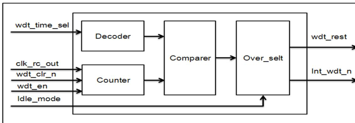
Due to the particularity of the system application, the watchdog timer overflow signal is classified:
