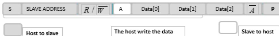
PS: T\_delay: Reserve slave interrupt time, generally 60us~300us, if the slave IIC interrupts the service processing time at 100us, suggest T\_delay>200us .
