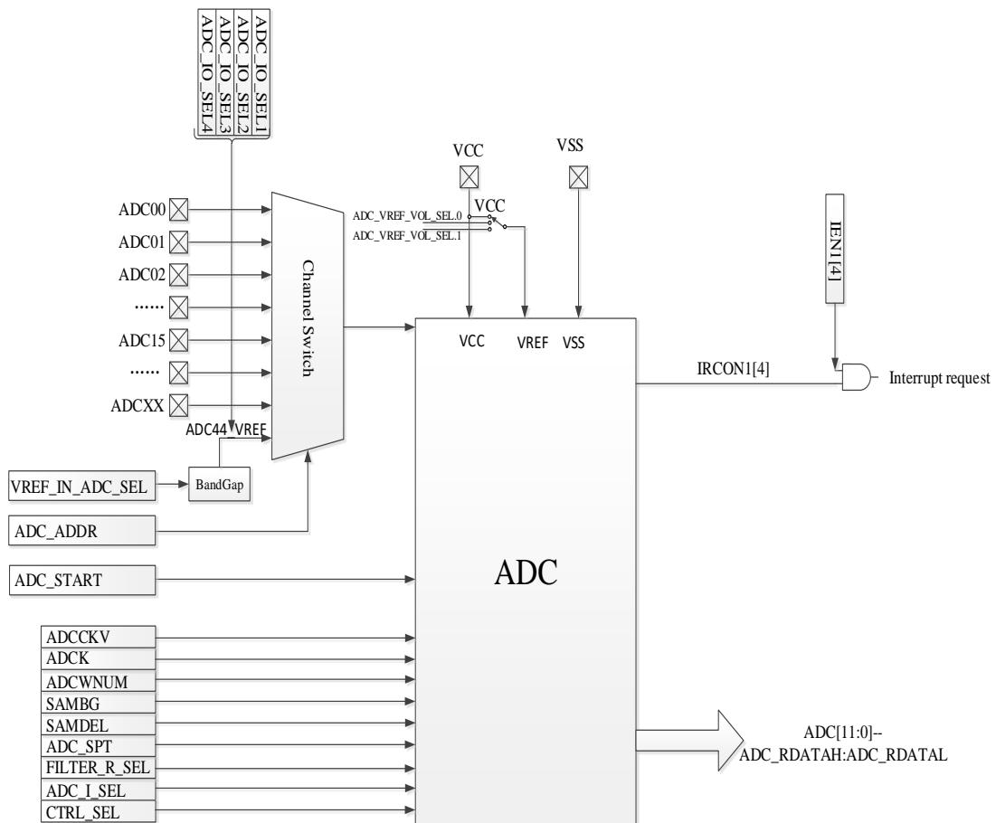
ADC structure block diagram
