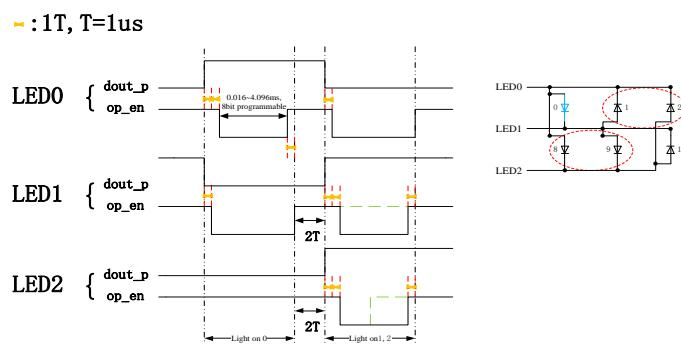
Note: 1. dout\_p: output data signal2. op\_en: output enable signal
