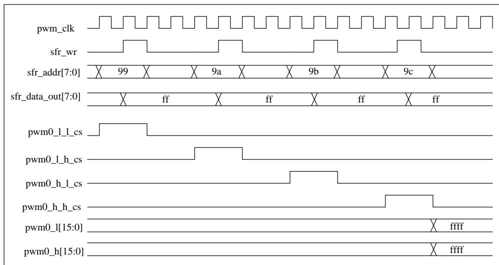
The period and pulse width of the PWM pulse width modulation module can be configured through registers. When  $PWM\_H + PWM\_L = 0$ , the output is low, but the configuration of the register must be selected when the PWM output port is valid (active high) and high. The high level control register and the low level control register must be configured in order from low to high, in order to ensure that the internal counter of the PWM module counts correctly and avoid generating wrong waveforms.
