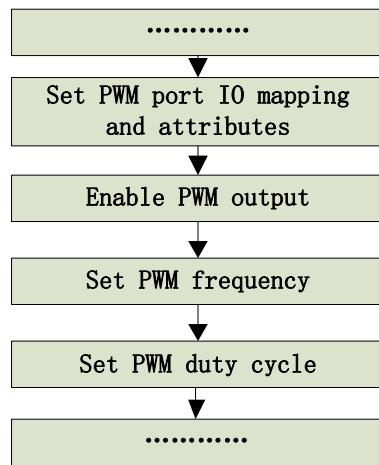
PWM Schematic diagram of configuration process
