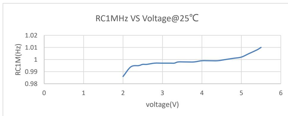
$f_{RC1M}$  voltage curve
