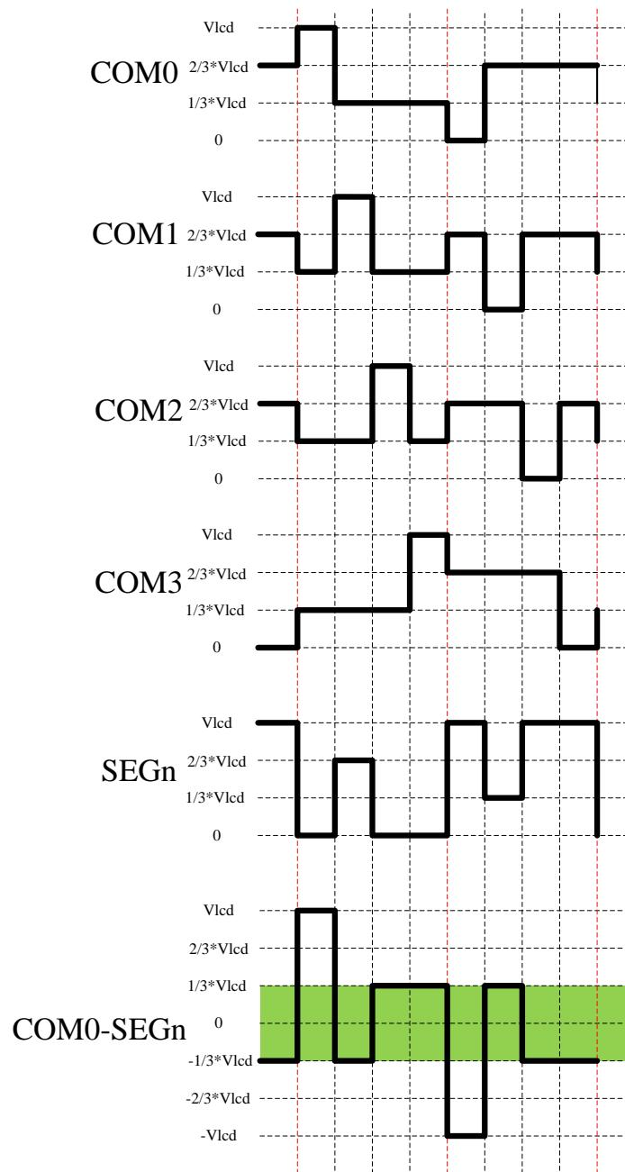
This realizes the bias voltage division sequence on the PAD, as shown in the figure below:
