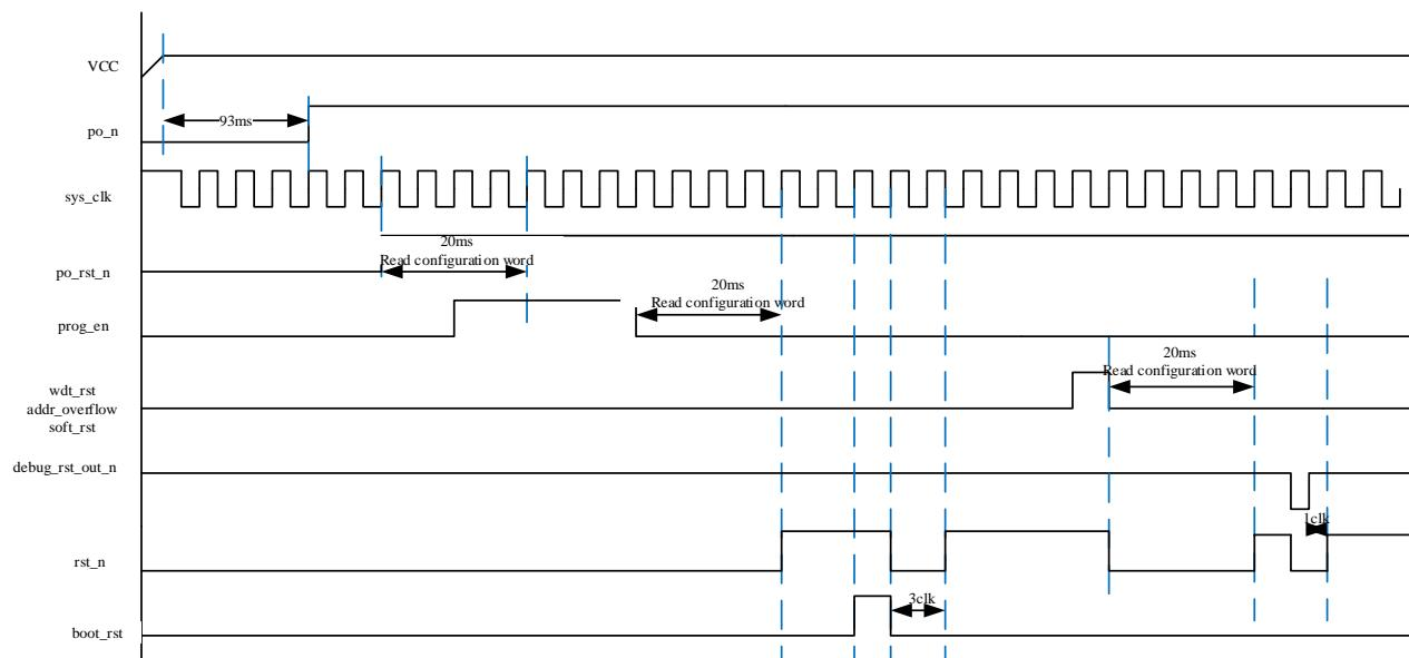
1. The chip has a power-on reset, and the analog POR module delays for 93ms, and po\_n is pulled high.
