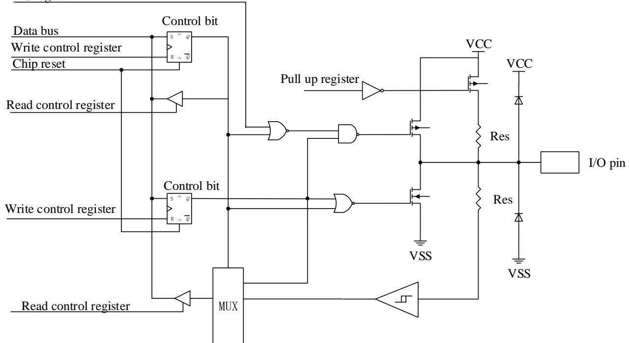
Open-drain output structure
