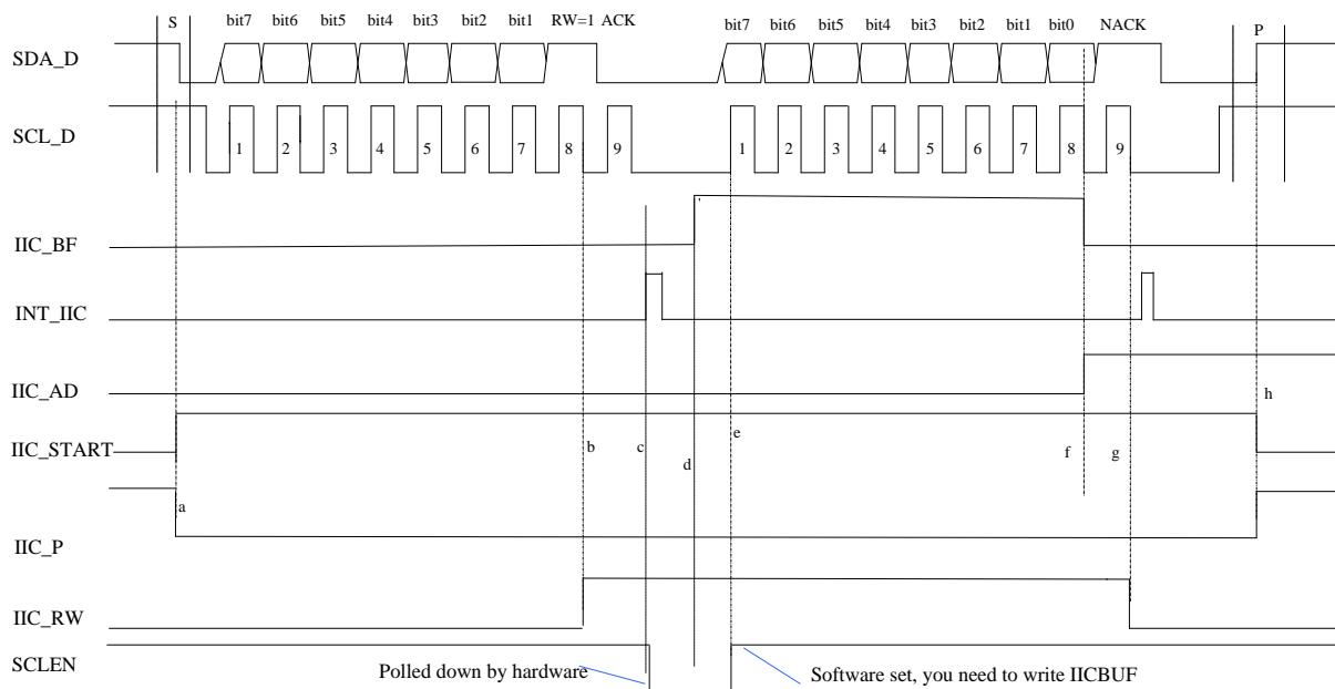
IIC host read pull low clock line diagram
